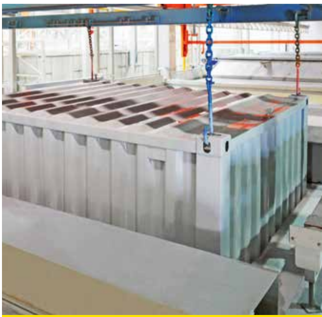
Zinc phosphatisation and cathodic electro dip paint primer
